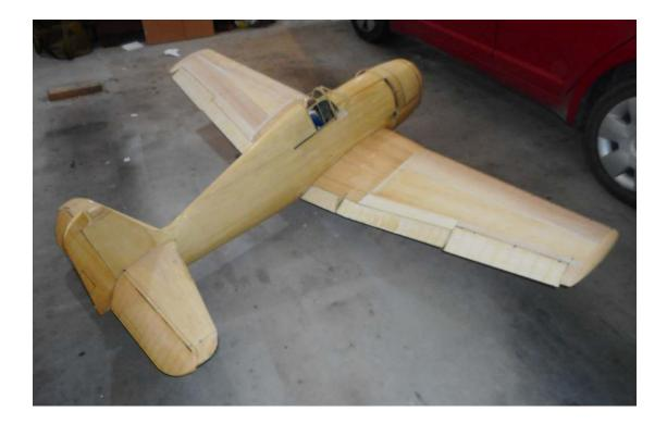
It is 1/6 scale and about 2.16 metre wingspan. With 50cc engine and retracts fitted it weighs 8.7kg, hopefully after finishing and painting and radio installation it will be about 10-11kg, not too bad for this type of model. Have fun, fly safely. (Carl M)
