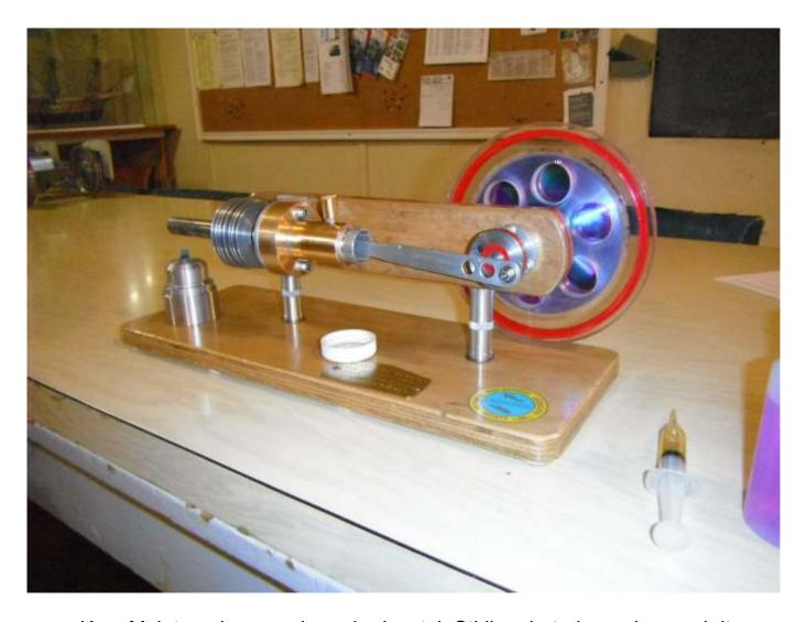
Ken McIntyre has made a horizontal Stirling hot-air engine and it was fascinating watching it operate. He had problems getting it going but determined that clearances between piston and cylinder were too neat. He added a lubricator for the piston using light machine grade oil which improved the situation markedly. There is a 50 deg C temperature difference between the ends of the heat exchanger.
