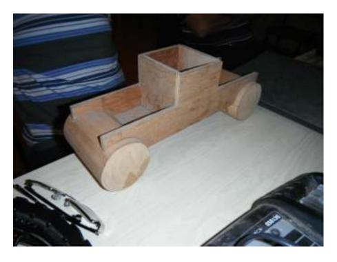
Lawrence Brehaut had brought along a mock-up of the cylinder unit for a 7 1/4" gauge NZR 'Q' loco and asked for advice on whether to fabricate the cylinders unit or to make a mould and cast as one piece. In discussion it was considered that fabricating cylinders and the surrounding structure and TIG welding together would be most practical. The cylinders could be bored and sleeved after welding.
