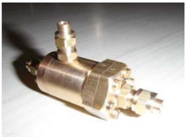
He also showed a triple valve he had made for the brake system. This is a simplified Westinghouse valve and is a form of fail-safe brake operating. There will be a triple valve on every bogey and a pneumatic reservoir. Nigel
